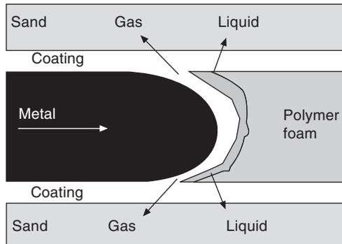
**Figure 15.3** An illustration of the transport of gas and liquid polymer degradation residues through STYROMOL and SEMCO PERM lost foam coatings.
